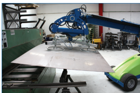
Intelligent load monitoring protects the operator and the load.
