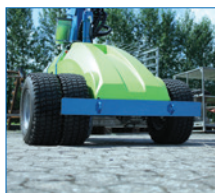
Twin wheels for rough terrain (optional)
