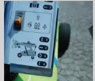
Wired remote control allows accurate placement of materials
