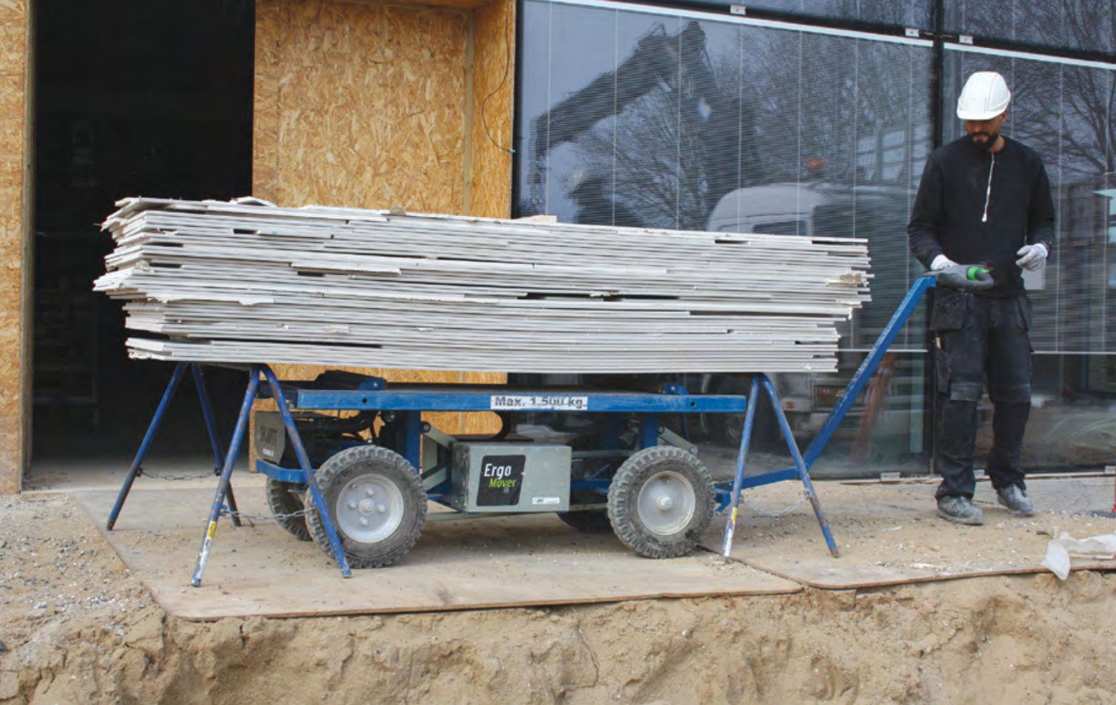
The ErgoMover Lift and Go can lift the platform 150mm, ideal for placing plasterboards on to trestles
