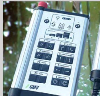
Operator-friendly design and integrated buttons make the multi-function control panel easy to use. Signal lights and double-action safety keys are included in the standard Winlet 375 set-up.
