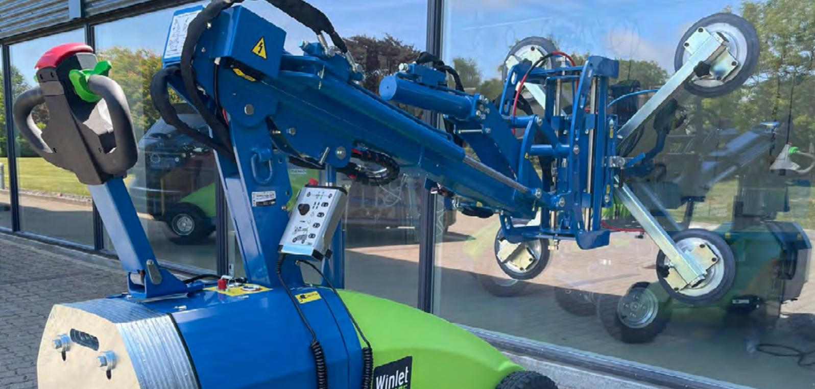
The Winlet 375 glazing robot minimises manual handling to maximise safety and productivity.
