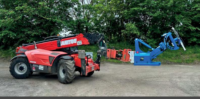
The Winlet 575TH has a hydraulic system which makes it independent from the telehandler
